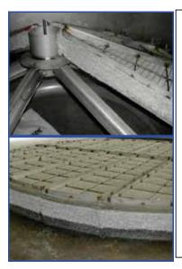
**Duty**: Removal of mist particles, in co-knitted fibre + demister mesh
