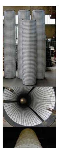
**Duty**: Removal of chemically or thermally generated sub-micron mists & fumes, using various design options.
