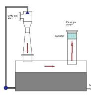
A high energy / high efficiency version of the Venturi uses a cyclone stage afterwards, and can remove 0.1 micron dust. It is not prone to blockage.
