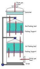
This design removes 2 different gases by absorption or by chemical reaction with different liquors with a dividing tray. Suitable for 1<sup>st</sup> stage 'stripping' and 2<sup>nd</sup> stage scrubbing.
