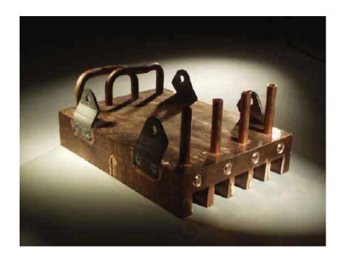
Copper cooling elements are a vital part of modern smelting technology.
