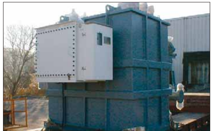
3200 KVA Furnace Transformer with OLTC
