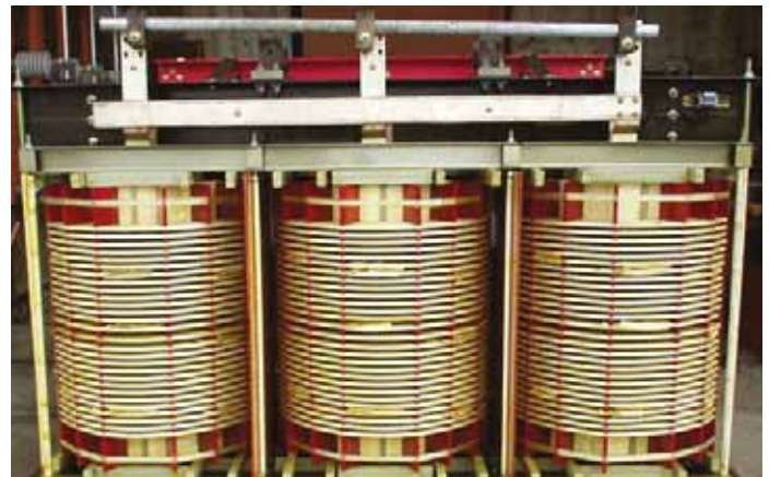
1500 KW 12 Pulse Traction Transformer at Short Circuit Testing Lab
