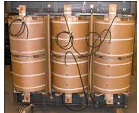
2100 KVA 12 Pulse Core & Oil
