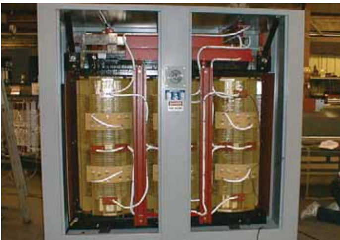
1400 KW 12 Pulse Traction Transformer
