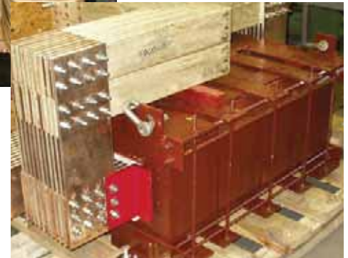
83 KA Interphase Transformer
