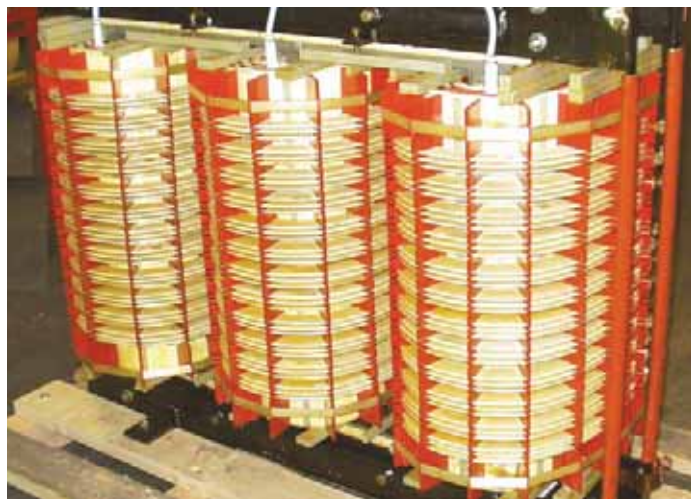
Drive Duty Transformer 24 Pulse
